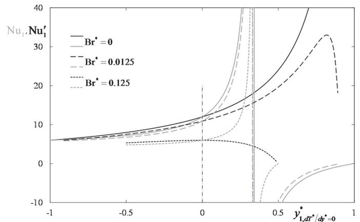
**Fig. 9** Nusselt number,  $Nu_1$ , versus the corresponding coordinate of the location of the temperature profile where  $\partial T/\partial y=0$ ,  $y_{1,dT^*/y^*=0}$ , for different values of the Brinkman number,  $Br^*$ , and  $n=0$ . Lines: Grey lines – “classical” approach, black lines - new approach, the vertical line marks the duct axis coordinate..
