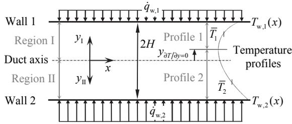
**Fig. 1** Schematic representation of the parallel plates duct, the boundary conditions and of the coordinate systems. A temperature profile is also shown, which is divided by the point where  $\partial T/\partial y=0$ .
