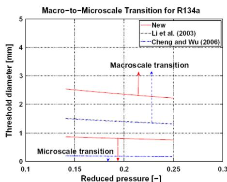
**Fig. 1** Transition criterion of Ong and Thome (2011a). “Reprinted from Experimental Thermal and Fluid Science, 35(1), Ong, C.L., and Thome, J.R., Macro-to-microchannel transition in two-phase flow: Part 1-Two-phase flow patterns and film thickness measurements, pp. 37-47 (2011), with permission from Elsevier.”
