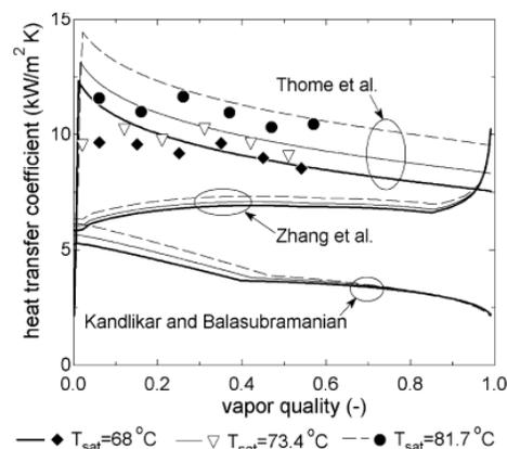
**Fig. 3** Comparison of the micro-scale prediction methods and the experimental data of Bao et al. (2000) (Ribatski et al., 2006). “Reprinted from Experimental Thermal and Fluid Science, 31(1), Ribatski, G., Wojtan, L., and Thome, J.R., An analysis of experimental data and prediction methods for two-phase frictional pressure drop and flow boiling heat transfer in micro-scale channels, pp. 1-19 (2006), with permission from Elsevier.”
