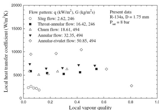
**Fig. 2** Flow boiling data of Saisorn et al. (2010). “Reprinted from International Journal of Heat and Mass Transfer, 53(19-20), Saisorn, S., Kaew-On, J., and Wongwises, S., Flow pattern and heat transfer characteristics of R-134a refrigerant during flow boiling in a horizontal circular mini-channel, pp. 4023-4038 (2010), with permission from Elsevier.”
