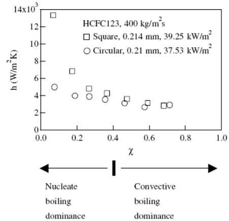
**Fig. 4** Heat transfer coefficient data for different shaped cross-sections of Yen et al. (2006). “Reprinted from International Journal of Heat and Mass Transfer, 49(21-22), Yen, T.-H., Shoji, M., Takemura, F., Suzuki, Y., and Kasagi, N., Visualization of convective boiling heat transfer in single microchannels with different shaped cross-sections, pp. 3884-3894 (2006), with permission from Elsevier.”
