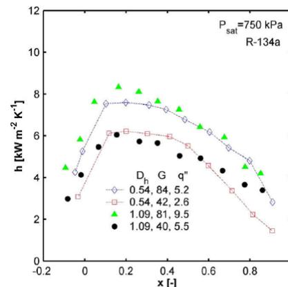
**Fig. 5** Heat transfer coefficient data for different hydraulic diameters of Bertsch et al. (2009a). “Reprinted from International Journal of Multiphase Flow, 35(2), Bertsch, S.S., Groll, E.A., and Garimella, S.V., Effects of heat flux, mass flux, vapor quality, and saturation temperature on flow boiling heat transfer in microchannels, pp. 142-154 (2009), with permission from Elsevier.”
